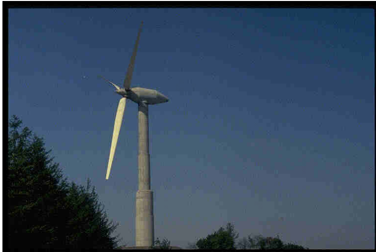
Fig. 1 Typical three blades wind turbine located in Denmark (rotor diameter 54m, 600 kW) A photo gallery available at : http://www.afm.dtu.dk/wind/turbines/gallery.html
