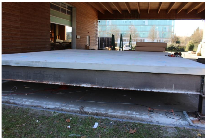
Figure 3.8: Side view of the floor specimen
