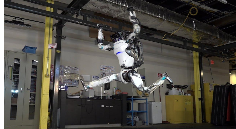
Atlas robot (Boston Dynamics) performing a sequence of dynamic maneuvers that form a gymnastic routine
