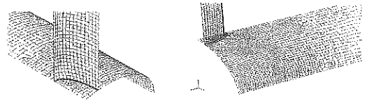
Figure 12. Modelling of the welds.
