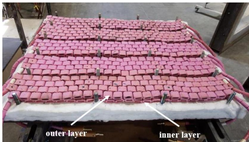
Figure 4. Positioning of two heating pads layers: outer layer and inner layer
