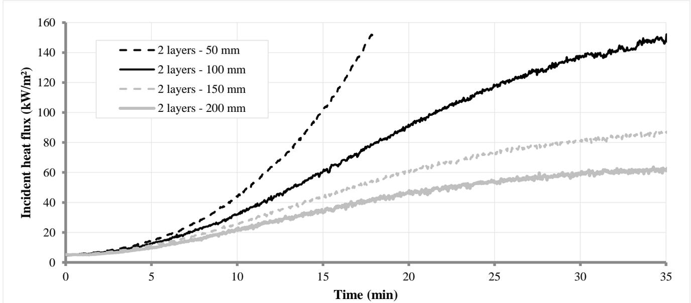
Figure 5. Incident heat flux obtained with two layers of heating pads, and for the distance of 50mm, 100mm, 150mm and 200mm between the heating pads and the specimen, with full power of the transformer
