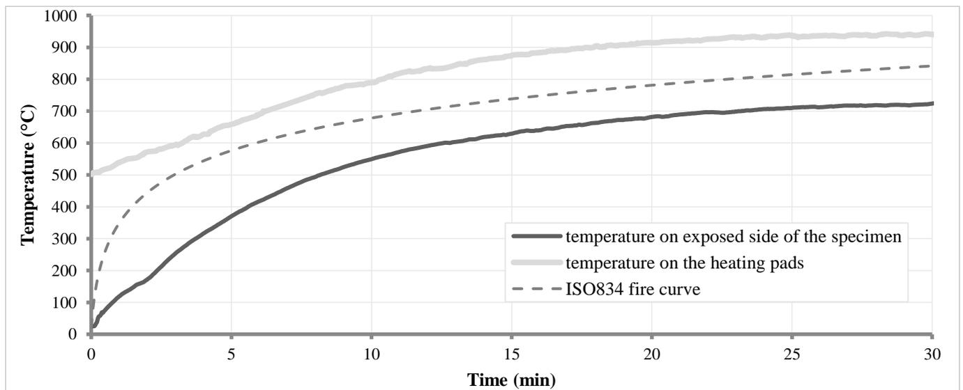
Figure 10. Temperature evolution on exposed side of the glass specimen, compared to temperature on the heating pads and the ISO834 fire curve
