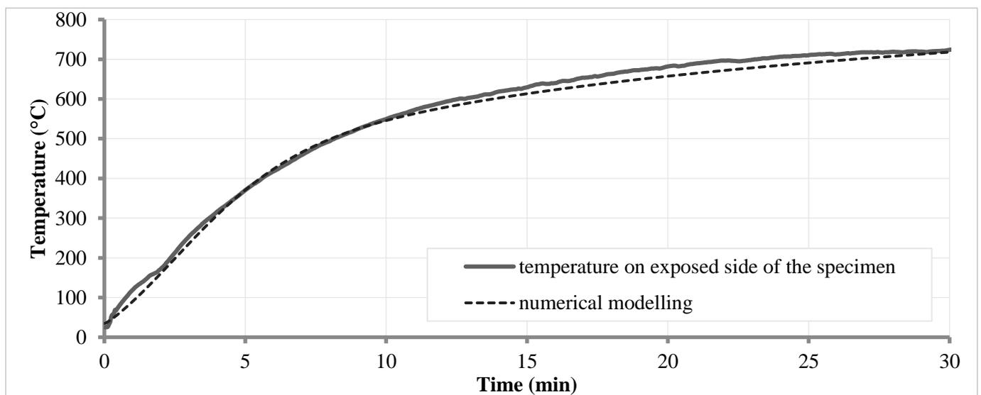
Figure 12. Temperature evolution on exposed side of the glass specimen obtained through numerical modelling and compared to experimental results
