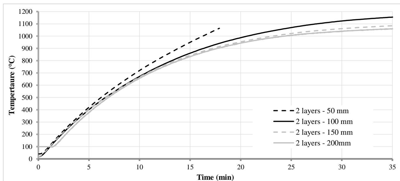
Figure 9. Temperature increase measured on the heating pads' surface for two layers of heating pads, and for the distance of 50mm, 100mm, 150mm and 200mm between the heating pads and the specimen, with full power of the transformer
