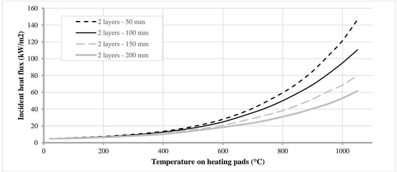
Figure 6. Incident heat flux dependence on temperature obtained on the heating pads for two layers of heating pads, and for the distance of 50mm, 100mm, 150mm and 200mm between the heating pads and the specimen, with full power of the transformer
