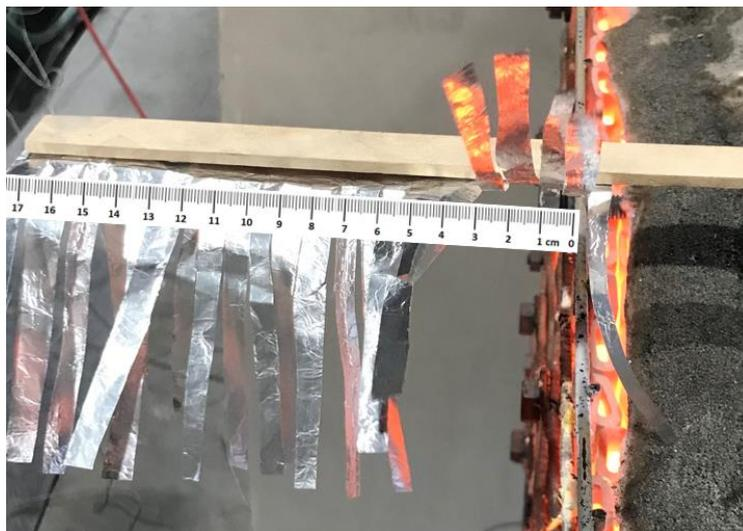
Figure 8. The zone of convective influence coming from the heating pads - qualitative measurement using a flag made of aluminium thin foil
