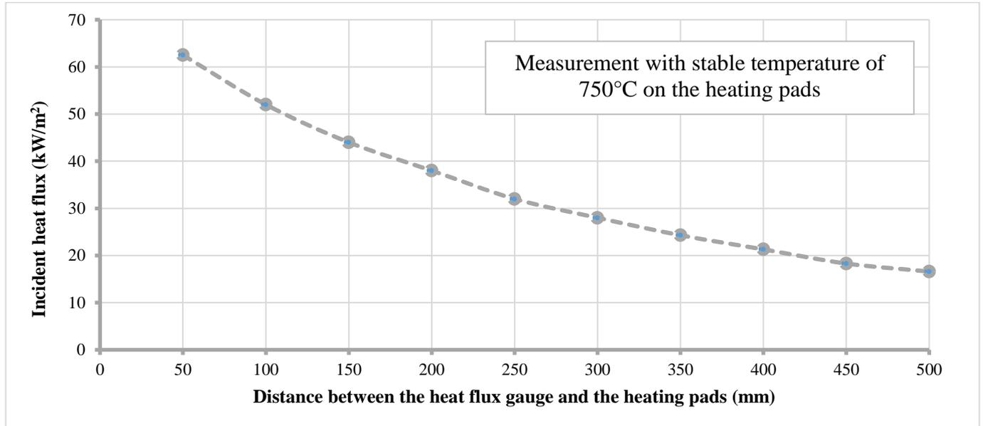
Figure 7. Incident heat flux obtained for different distance between the heating pads and the specimen, with two layers of heating pads, for stabilized temperature on the heating pads of 750°C
