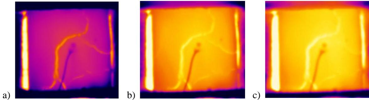
Figure 11. Temperature distribution on the unexposed side of the glass sample, captured by infrared camera for different temperatures on unexposed side: a) 350°C, b) 475°C, c) 550°C
