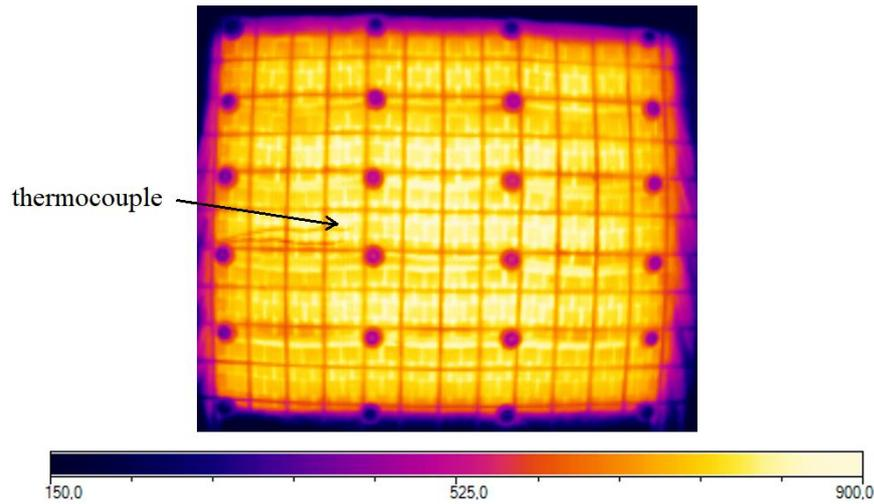
Figure 3. Temperature distribution on the heating pads, captured by infrared camera for temperature 800°C measured by the thermocouple in the centre of the heating pads
