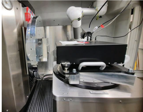
Figure 3 : Implementation of the deflector on the B-axis baseplate of the 350FG lathe
