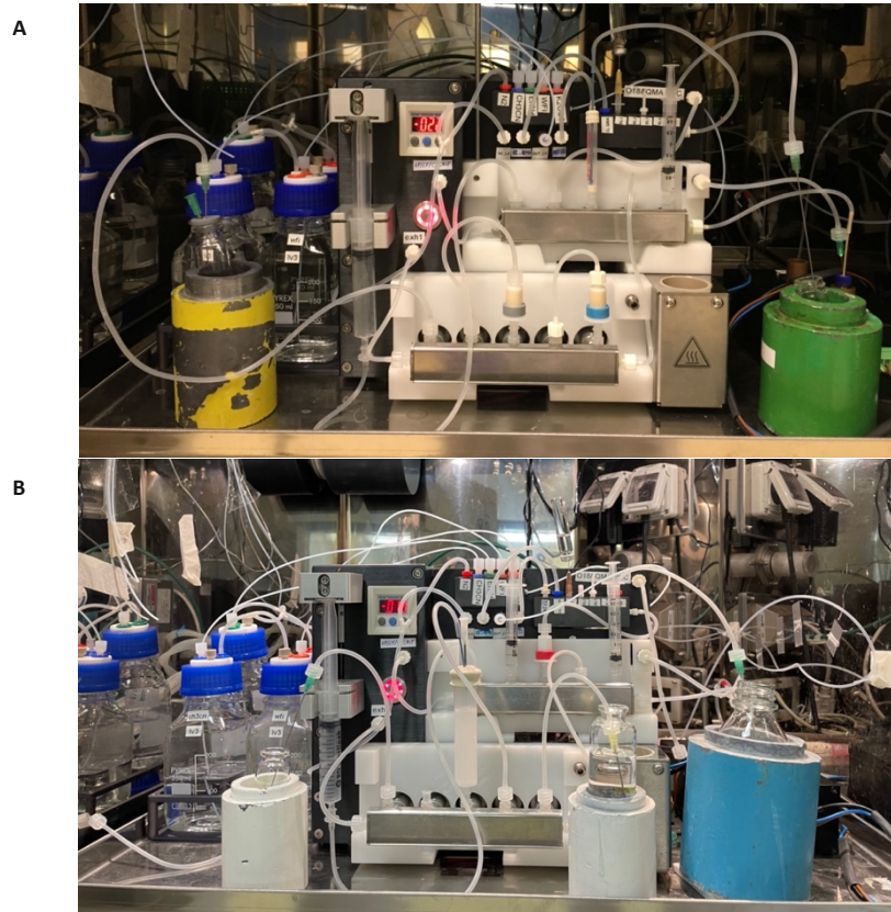
Figure S1. Radiosynthesizer for the synthesis of (A) [ ^{18}\text{F} ]SFB and (B) [ ^{18}\text{F} ]SFB-nanobody.
