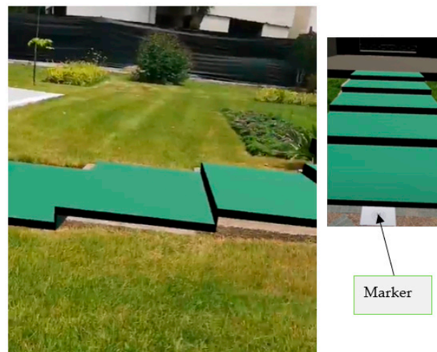
Figure 14. 3D model placement using ARcore SDK (Anchor method).
