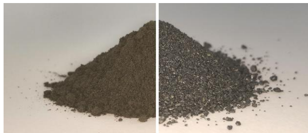
Fig. 7. The metallic product (right) produced from lunar regolith (left, regolith simulant)
