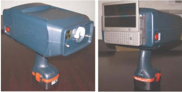
Fig. 4. Handheld instrument with miniature X-ray tube
