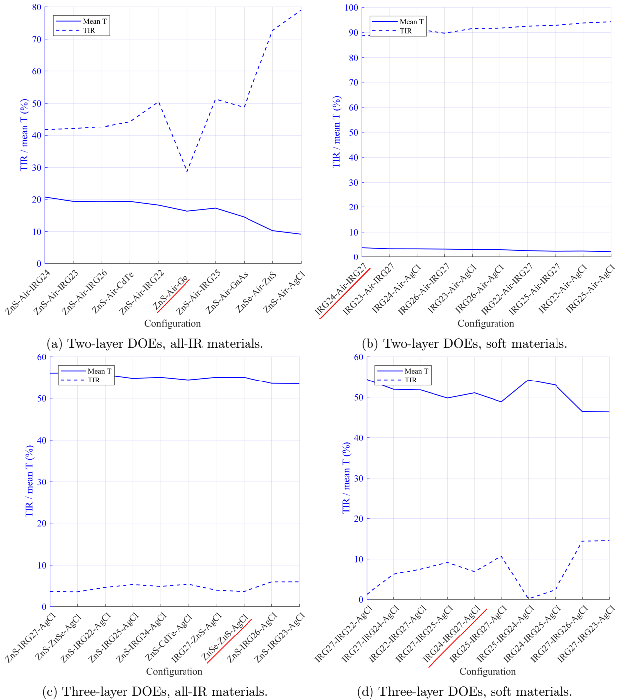
Figure 11.9: Off-axis geometric selection method results for the ten "best" material configurations considering: a) Two-layer DOEs, all-IR materials, b) two-layer DOEs, soft materials, c) Three-layer DOEs, all-IR materials, d) three-layer DOEs, soft materials. The same materials and x-label configuration have been kept from Figures 11.5 and 11.6 to ease the comparison. The design parameters are D = 10 mm, F/15 and N = 10 . Three evaluation metrics are shown: transmission (blue line, left axis), TIR (blue dotted line, left axis) and thickness (black line, right axis). The "best" MLDOE combinations selected in Figures 11.5 and 11.6 are underlined in red.
