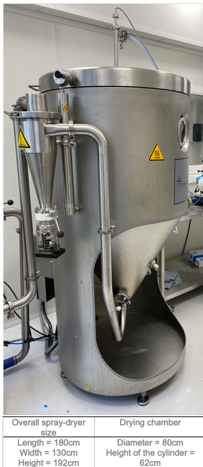
Figure I-25: Picture of the GEA Niro Mobile minor spray-dryer used in this work and overall dimension of the equipment.
