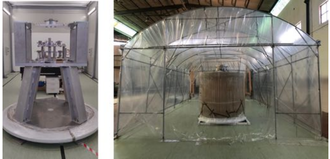
Figure 17. Left: Picture of the final setup (still under construction) positioned on a solid table grounded to the cryostat basis. It is positioned inside the Archimedes hangar. Right: Tent structure hosting the cryostat cover.
