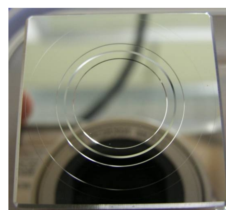
Fig. 10: 1 st result of the diamond turning of the refractive part
