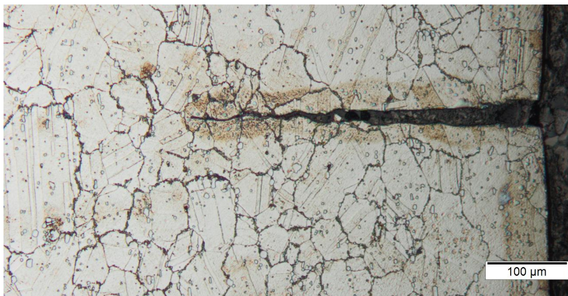
Figure 1.12 – Transgranular crack in the sample after anisothermal creep-fatigue testing
