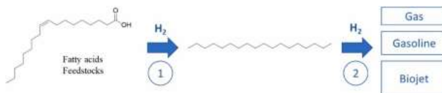
Fig. 9. Simplified hydro-processed esters and fatty acids (HEFA) into biofuels production process; 1) Hydrodeoxygenation and hydrogenation; 2) Hydrocracking and isomerization of long chain hydrocarbon into suitable biofuels (based on Karatzos et al., 2014) [23].
