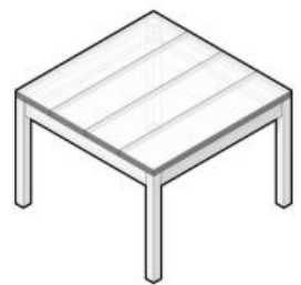
Glue-laminated columns and beams with cross-laminated timber floor panels
