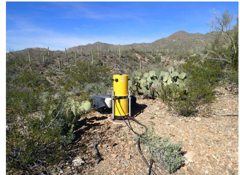
Groundwater storage studies using USGS A10 absolute gravimeter, [b]
