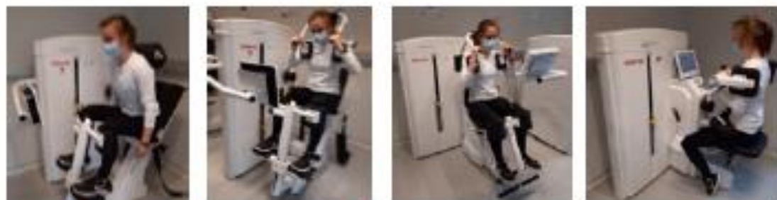
Figure 1 : David Back Dynamometers (David International Ltd., Vantaa, Finland) for trunk extension, flexion, rotation and lateral flexion respectively.
