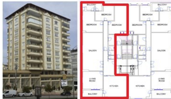
Fig. 1: A general view and floor plan of the selected building (Atmaca and Atmaca, 2015).
