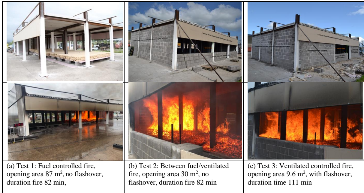
Figure 2: Different opening layouts were used for the three tests
