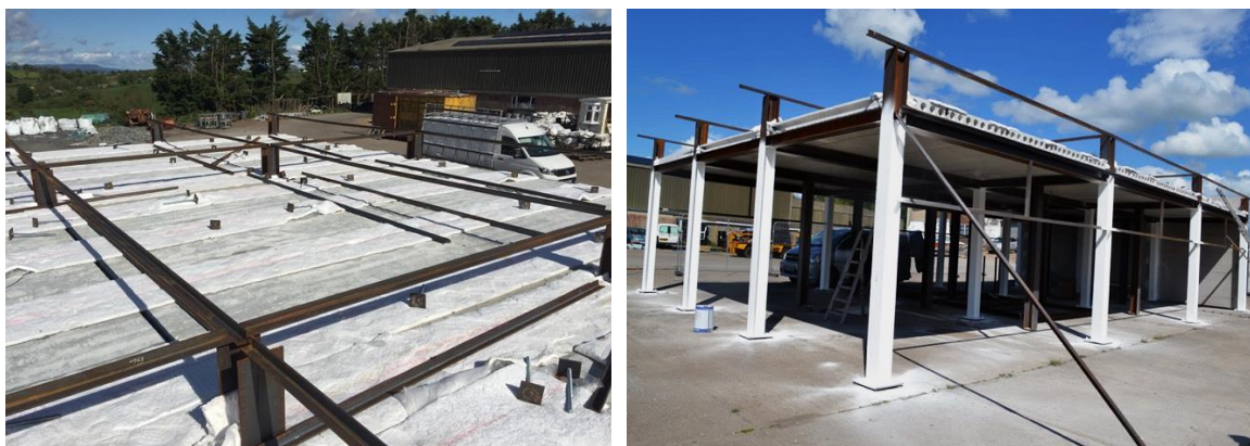
Figure 21: The fire blanket used to protect the cables of instrumentation (left) and the protected columns of the test compartment (right)
