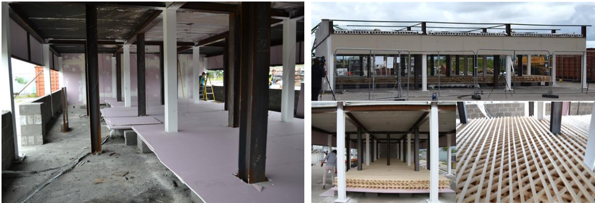
Figure 22: Platform for laying of fuel wood (left) and fuel wood arrangement used during the three large-scale tests (right)
