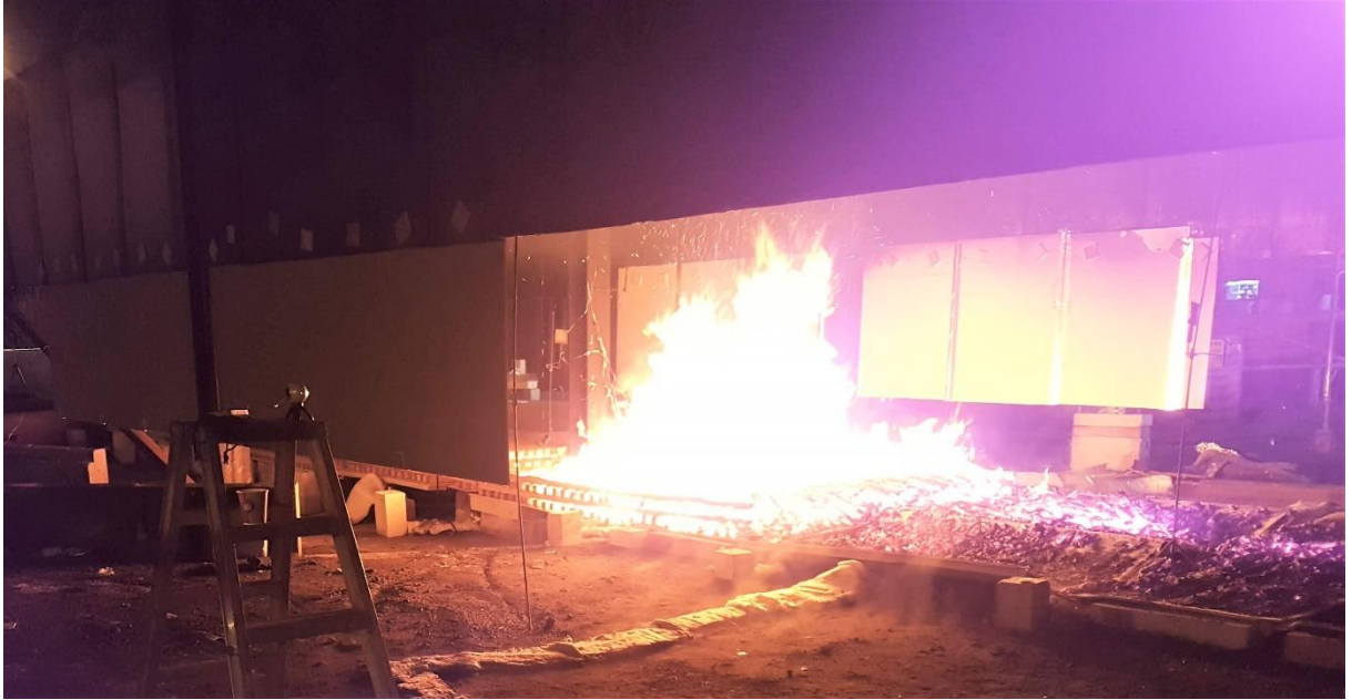
Figure 17: Photo of the wood crib experiment showing the travelling fire
