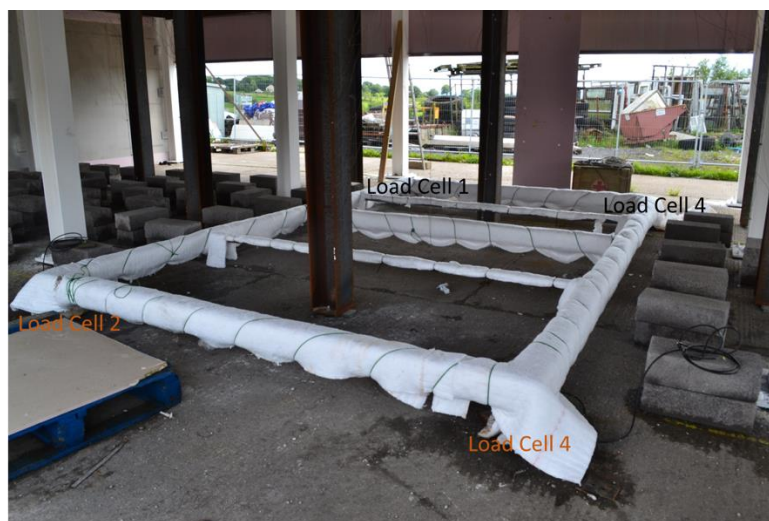
Figure 77: Preparing the steel platform for the mass loss recording (4 load cells)
