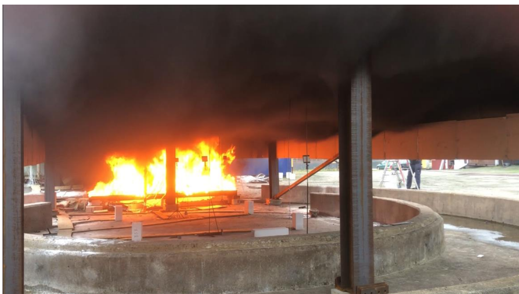
Figure 15: Photo showing the clearly defined smoke layer in the diesel pool fire tests
