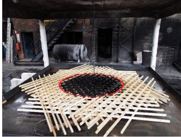
Figure 13: Isotropic fire propagation after the upper layers of sticks have been removed
