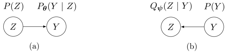
Figure 4.4: The description of a variational auto-encoder with Bayesian networks. (a) The decoding process samples the latent variables from P(Z) and generates observations Y by sampling conditionally from P_{\theta}(Y | Z) . (b) The encoding process takes an observation from the dataset Y \sim P(Y) and computes the approximate posterior Q_{\psi}(Z | Y) corresponding to the model in (a) .
