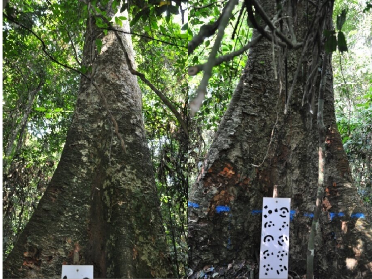
Fig. S2.1: Focal buttressed trees with surrounding vegetation that limits the photogrammetric process. The white panel is a panel with coded targets which are automatically detected by the photogrammetric software Photoscan.
