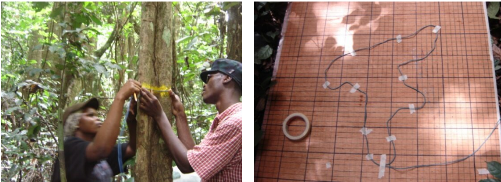
Figure 1.5: Wire method to estimate the basal area of a cross-section (left: shaping the wire, right: counting the number of squares with a reference area).
