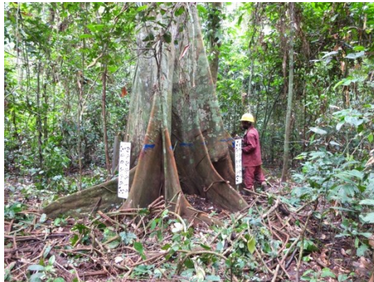
Fig. S2.2: Focal buttressed tree with the small vegetation and the liana removed. Four panels with coded targets were positioned in the four cardinal points to add artificial tie-points in the photogrammetric process. The panel from the south was used as the metric reference (one vertical line of the coded target was considered as the z axis). The distance between the highest coded targets of the reference panel and the ground was measured to deduce the height of the coded targets.
