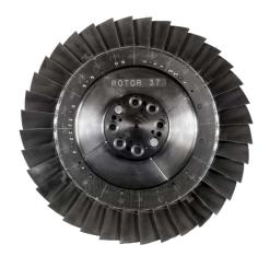
FIGURE 4.1 – Picture of NASA rotor 37 [95].
