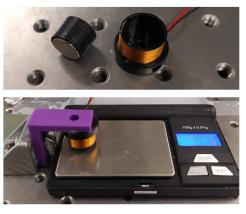
Figure 6: Force output of the custom voice-coil actuator fed with DC current (left) and experimental setup (right). The voice-coil was mounted on a scale and fed with DC current. The weight reading on the scale can be upconverted to a force reading measurement. The force constant of 0.6465 N/A have been measured.
