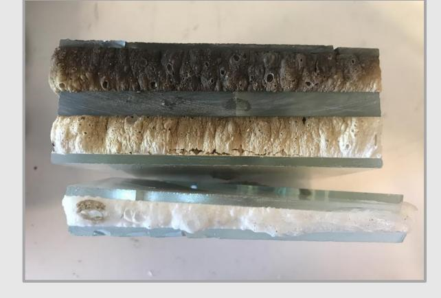
Besides all properties of the intumescent layer, the change in volume (swelling) should also be taken into account. This phenomena was integrated in the effective thermal properties applied in the model considering the initial thickness of gel and the thickness of foam layer after the reaction has finished. be further analyzed.
