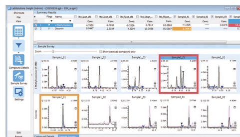
Simultaneous analysis of 434 pesticides using Smart SIM
