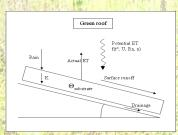
We established a model concerning three types of green roofs and a flat roof storage system based on a physical approach. The water balance's terms were estimated: evapotranspiration depending on vegetation layer (sedums, grass, shrubs, trees...), runoff and interflows (via hydraulic conductivity, albedo)... The hourly meteorological data were recorded at Ernage (Namur, Belgium) and covered 7 years (1989-95). The
