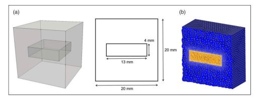
**Figure 5:** Representation of the experimental setup simulated to perform numerical validation of the developed model and evaluate parallel performance. (a) A cuboid of Mg (with the size of  $13 \text{ mm} \times 13 \text{ mm} \times 4 \text{ mm}$ ) is floating inside a simulated body fluid solution to investigate the degradation process, and (b) a cross-section of the computational mesh, refined on the metal-medium interface to increase the interface capturing accuracy.
