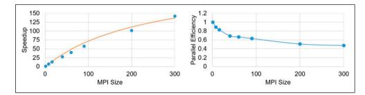
Figure 11: Speedup and parallel efficiency of the strong-scaling experiment. The orange line in the left plot is the fitted equation based on the Amdahl rule.
