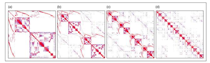
Figure 4: Comparison of the sparsity patterns (highlighting non-zero elements) of the global matrix A for a different number of decomposed domains: (a) I domain, (b) 2 sub-domains, (c) 4 sub-domains, and (d) 8 sub-domains.
