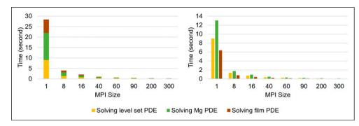
Figure 10: Strong-scaling test result. Results are broken down into contributions for each PDE, which are plotted cumulatively and separately in the left and right plot, respectively.
