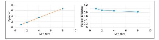
Figure 9: Speedup and parallel efficiency of the weak-scaling experiment. The orange line in the left plot shows the fitted curve based on the Gustafson equation.
