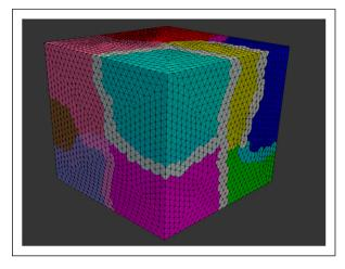
Figure 3: Overlapping domain decomposition in the current study. Each color shows a separate sub-domain, and the narrow lighter bands are the overlapped regions.
