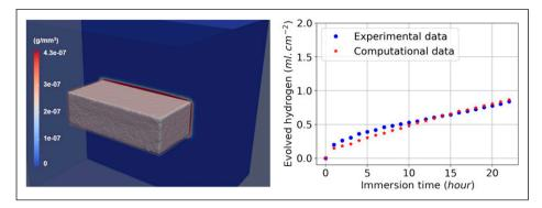
**Figure 7:** Numerical simulation result. Left: formation of a protective layer on the surface of the Mg block (red region). Right: comparison of the produced hydrogen (a surrogate for the material loss) in the computational model and the experimental data, which is a validation of the full model as both the reaction–diffusion equations and the level set equation are involved in the computation of this quantity.
