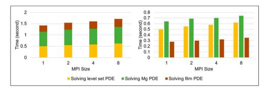
Figure 8: Weak-scaling test result. Results are broken down into contributions for each PDE, which are plotted cumulatively and separately in the left and right plot, respectively.
