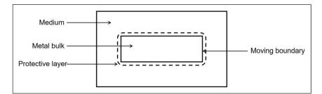
Figure 1: A schematic representation of different components of the developed model for simulation of the degradation process with a moving front.
