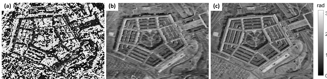
Fig. 4.7 Results of the pure phase object reconstruction: (a) conventional in-line reconstruction; (b) conventional off-axis reconstruction and (c) reconstruction using the proposed method.
