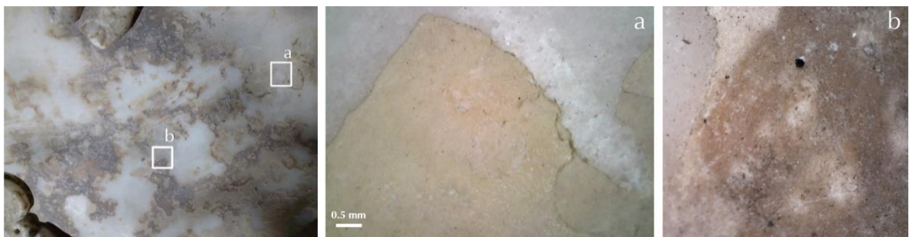
Figure 5. Lycian Apollo (MSR, RA172). Detail of the areas of the micrographs of the superficial polychromy (2nd phase): (a) multi-layered white paint; (b) grey-brown paint on the white layer (same scale).
