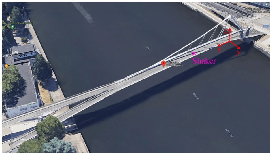
Figure 5: Photo of the “La Belle Liégeoise” footbridge. The frame of reference and the location of the shaker are also indicated. (Image from Google Maps.)
