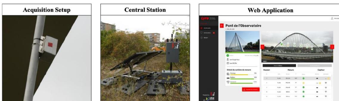
**Figure 2:** the LYRA solution, comprising wireless sensors (left), a central station (middle) and a cloud solution (right)
