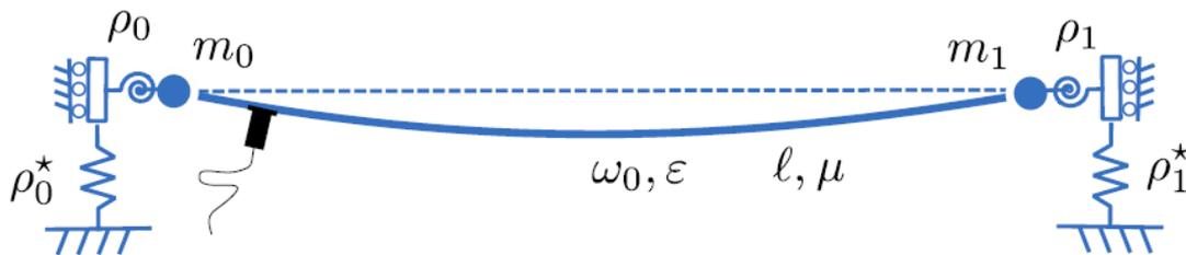
**Figure 3:** Parametric model of a cable
