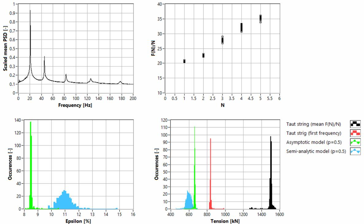
**Figure 10:** Identification results on stay 2 of the Harchies bridge (311 measurements from 31/01/2020 to 11/03/2020)
