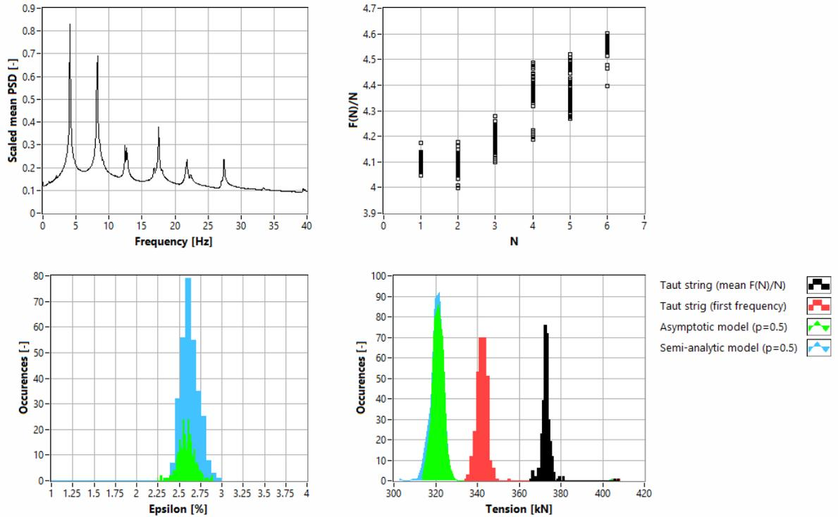
**Figure 9:** Identification results on stay 15 of the Observatoire bridge (304 measurements from 06/12/2019 to 03/01/2020)
