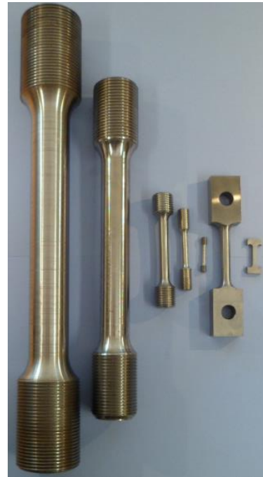
Variety of specimens for tensile testing of different dimensions
