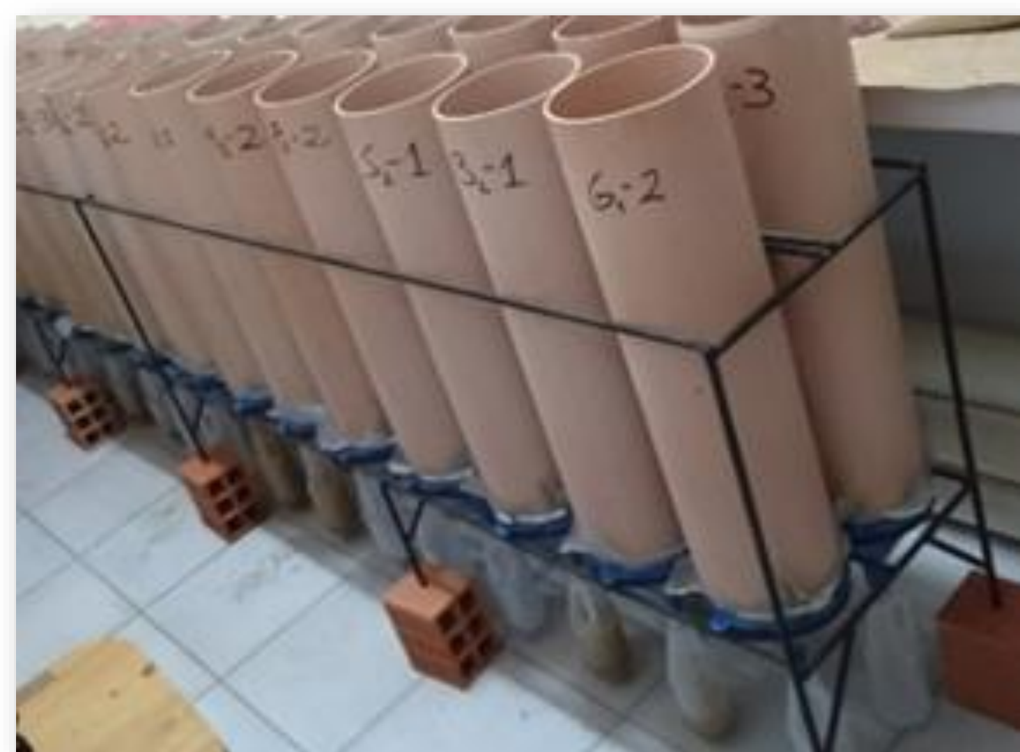
Fig 1. Experimental soil columns.
