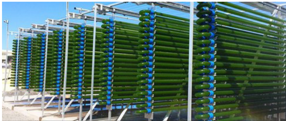
Figure 1.5 – Schematic representation of different types of photobioreactors (a): (A): vertical tubular, (B): helical tubular, (C): horizontal tubular, (D): flat panel, (E): airlift, (F): accordion type, (G): stirred tank, (H): bubble column. Reproduced from (Khetkorn et al., 2017) with authorization. Photography of industrial tubular reactors (b). A Varicon Aqua Phyco-Flow serpentine photobioreactor growing Haematococcus pluvialis in Kona, Hawaii. Image courtesy of Varicon Aqua Solutions Ltd. UK (2018) (Varicon Aqua Solutions, n.d.).
