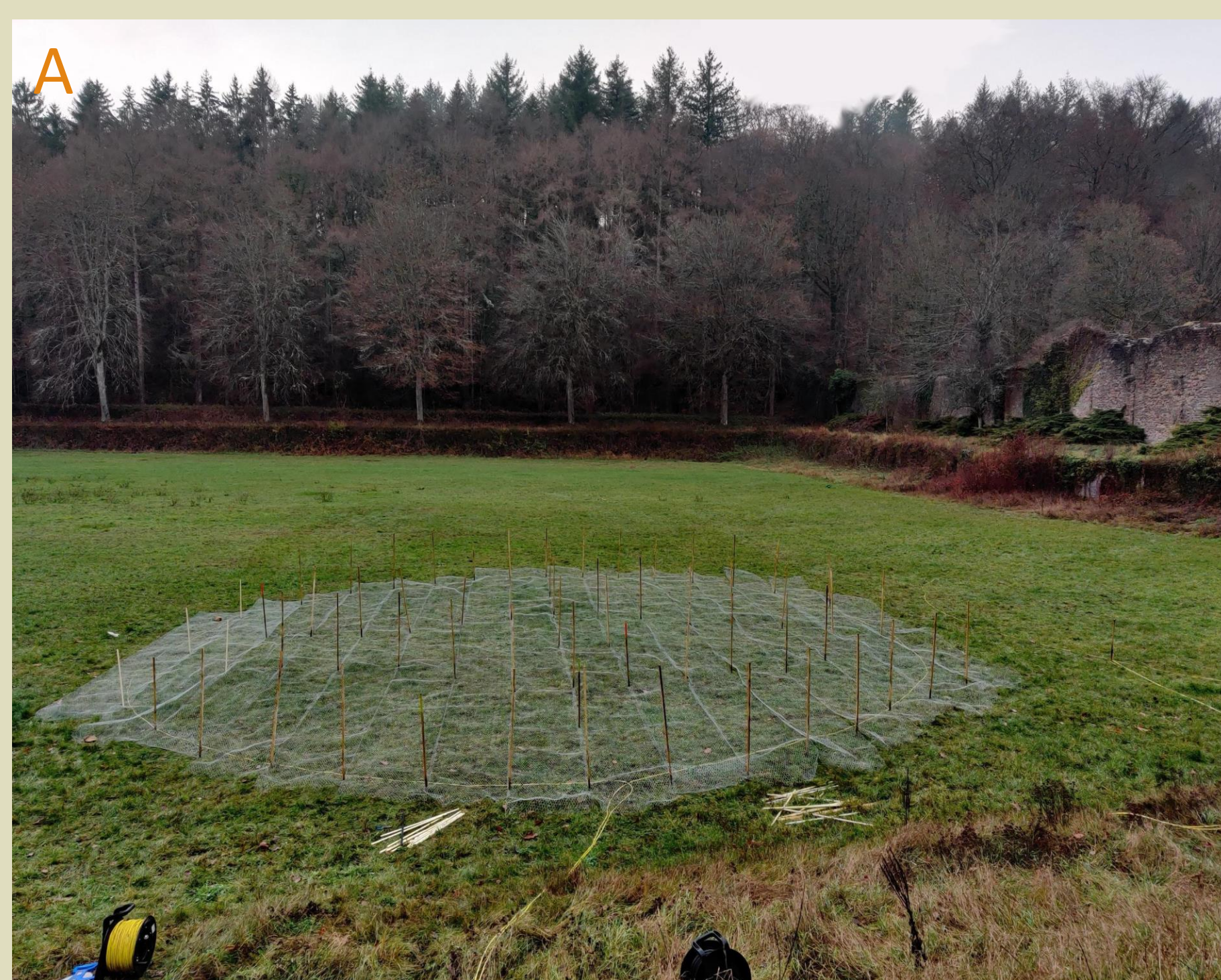
Figure 2: Pictures of different tested filtering dispositions. (A) Dome built above the antenna loop. (B) ERT line on the test site with the Orval Abbey in the background. (C) Tunnel built above the cable of the antenna loop.
