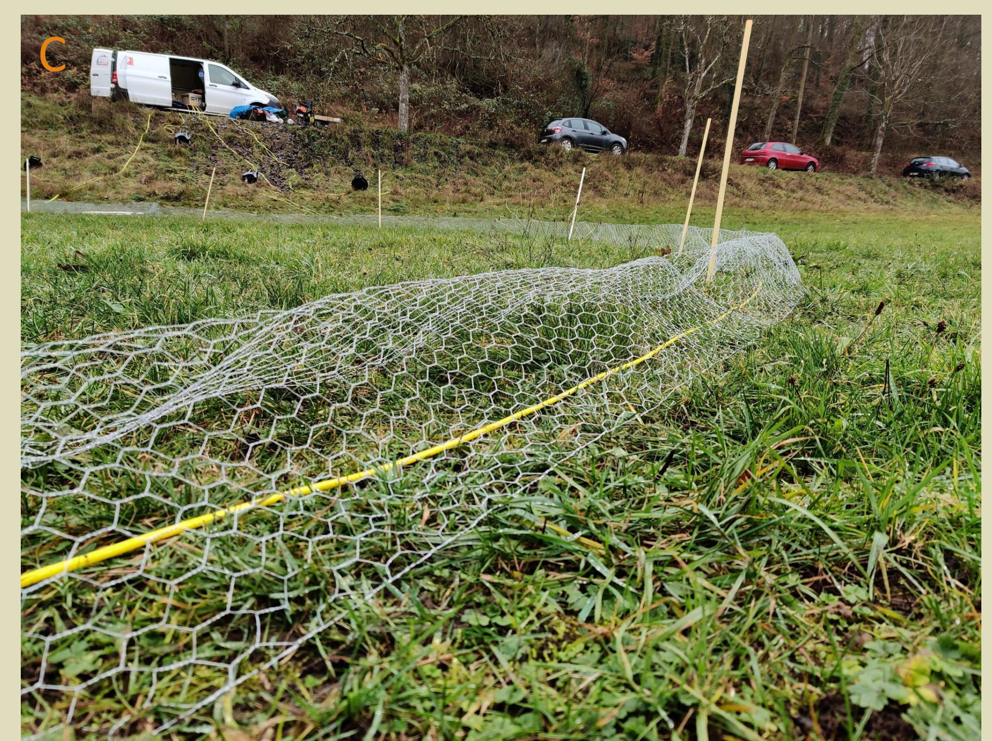
Figure 2: Pictures of different tested filtering dispositions. (A) Dome built above the antenna loop. (B) ERT line on the test site with the Orval Abbey in the background. (C) Tunnel built above the cable of the antenna loop.
