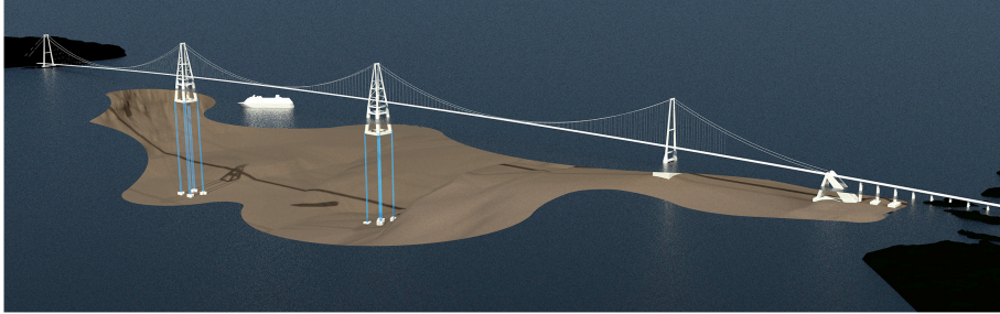
FIGURE 1: A three-span suspension bridge with tension-leg platforms as pylons, one of the proposed floating bridge concepts for crossing the Bjørnafjorden strait in Norway. Illustrated by Arne Jørgen Myhre, Statens Vegvesen. Courtesy of [15].
