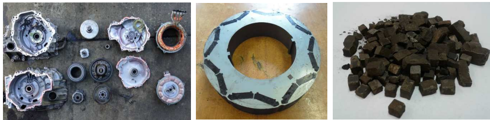
Manual dismantling and recovery of NdFeB magnets after thermal demagnetization
