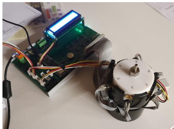
Figure 3 : Prototype of breath sensing gas sensor array used for benchmark building, nicknamed SAMBRE_1
