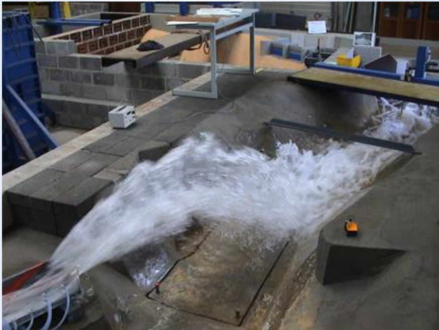
Sarrans Dam bottom outlet (France) – 1:35 scale model (left) and prototype (right) (Ercicum et al., 2020) #IAHRonlineforum
