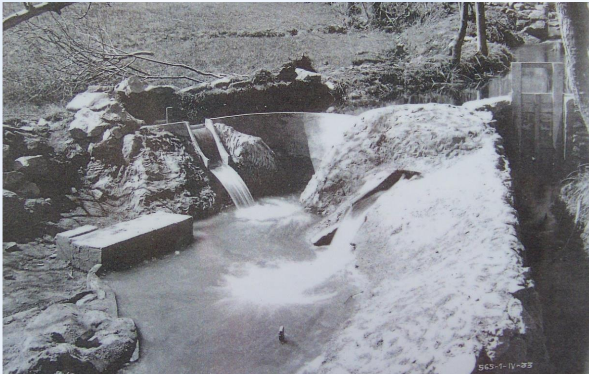
Marèges Dam (France) physical model built in 1933 close to the dam construction site (Erpicum S., Crookston B. et al., 2020)
