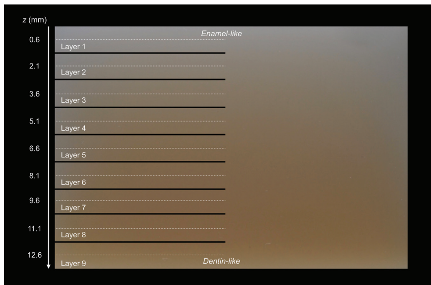
Fig. 1 A functionally graded polymer-infiltrated ceramic network (FG-PICN) block with, on the left part, a schematic illustration of the cutting into 9 layers from the top (enamel zone) to the bottom (dentin zone). The black spaces between the layers represent the 0.3 mm of material lost during cutting (saw thickness). The thickness of each layer is (1.2 \pm 0.1) \text{ mm} ; measurements refer to the center of each layer (dashed line).
