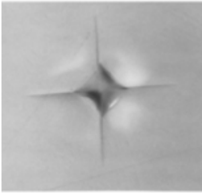
Figure 7. A Vicker's indentation with projecting cracks performed on a sample of a ceramic. The figure was reprinted from Sehgal and Ito (1998) with permission from John Wiley & Sons-Books
