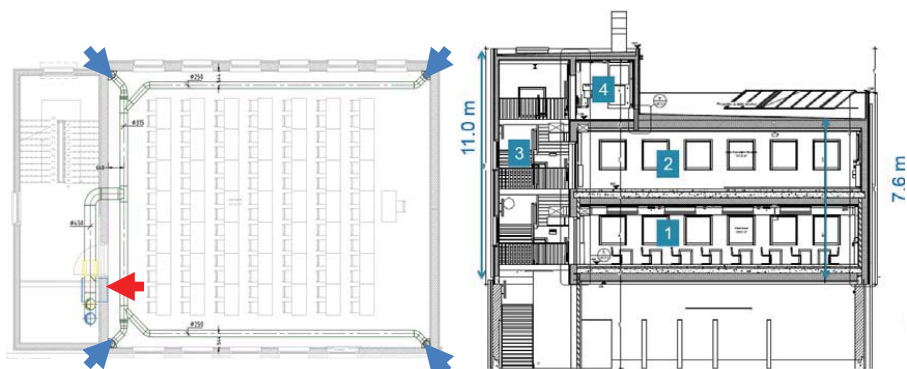
Figure 2; (Left) Floor plan of the lecture room evaluated, blue is supply air and red extract air (Right) Cross-section of the building (1) lecture room (2) lecture room (3) staircase (4) technical room
