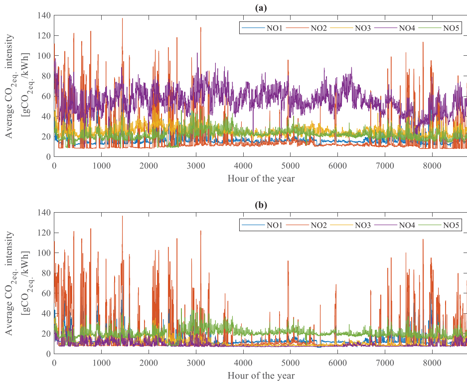
Figure 2: Hourly average CO_{2eq.} intensity of the electricity mix in Norwegian bidding zones for (a) Scenario 1 and (b) Scenario 2.
