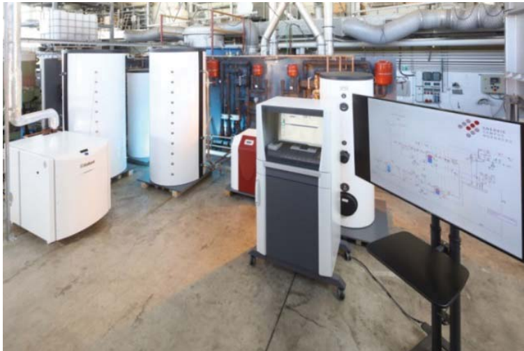
Figure 19: Emulation test bench - THN-Rednitzhembach
