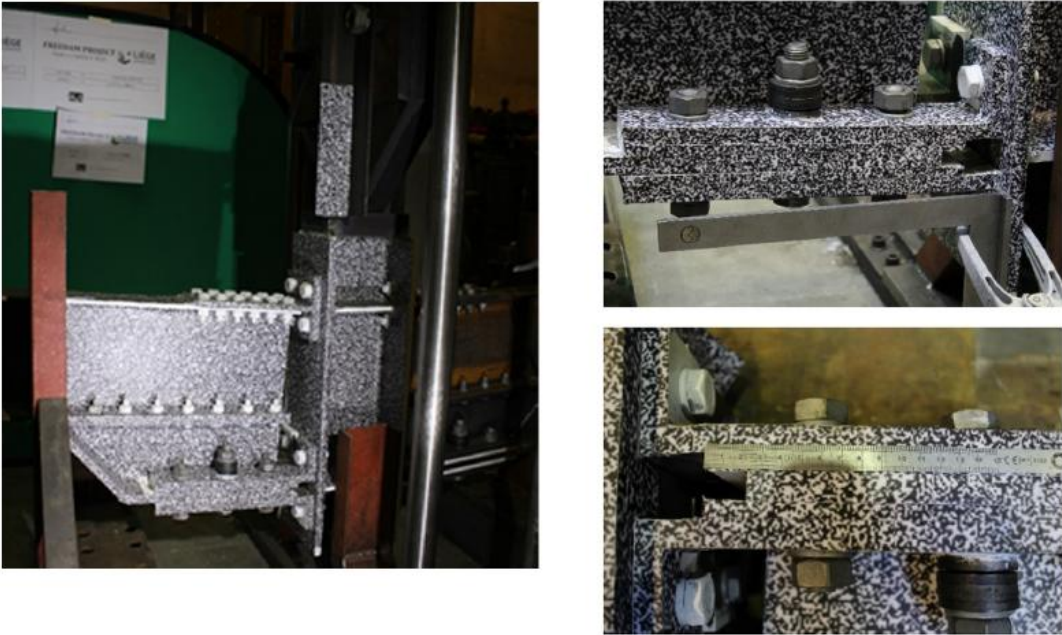
Fig. 9. Impact test results ITFR 06 M2 H3785 – slippage of the friction device.
