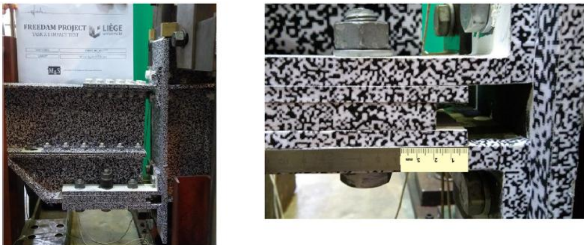
Fig. 8. Impact test results ITFR 02 M1 H4300 – slippage of the friction device.
