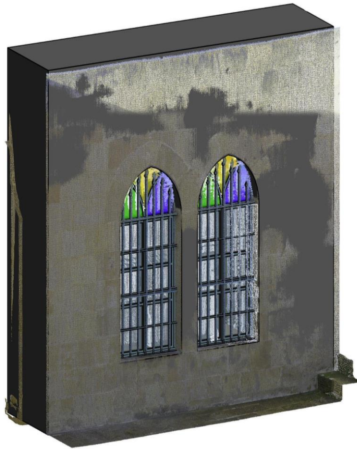
Figure 6. Axonometric overview of the BIM object with the associated point cloud
