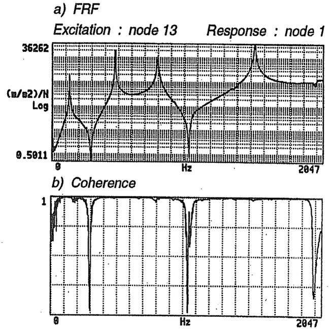
Fig. 7: Measured FRF and coherence function.
