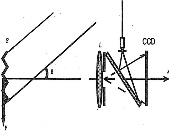
Fig. 2: Out-of-plane sensitive interferometer
