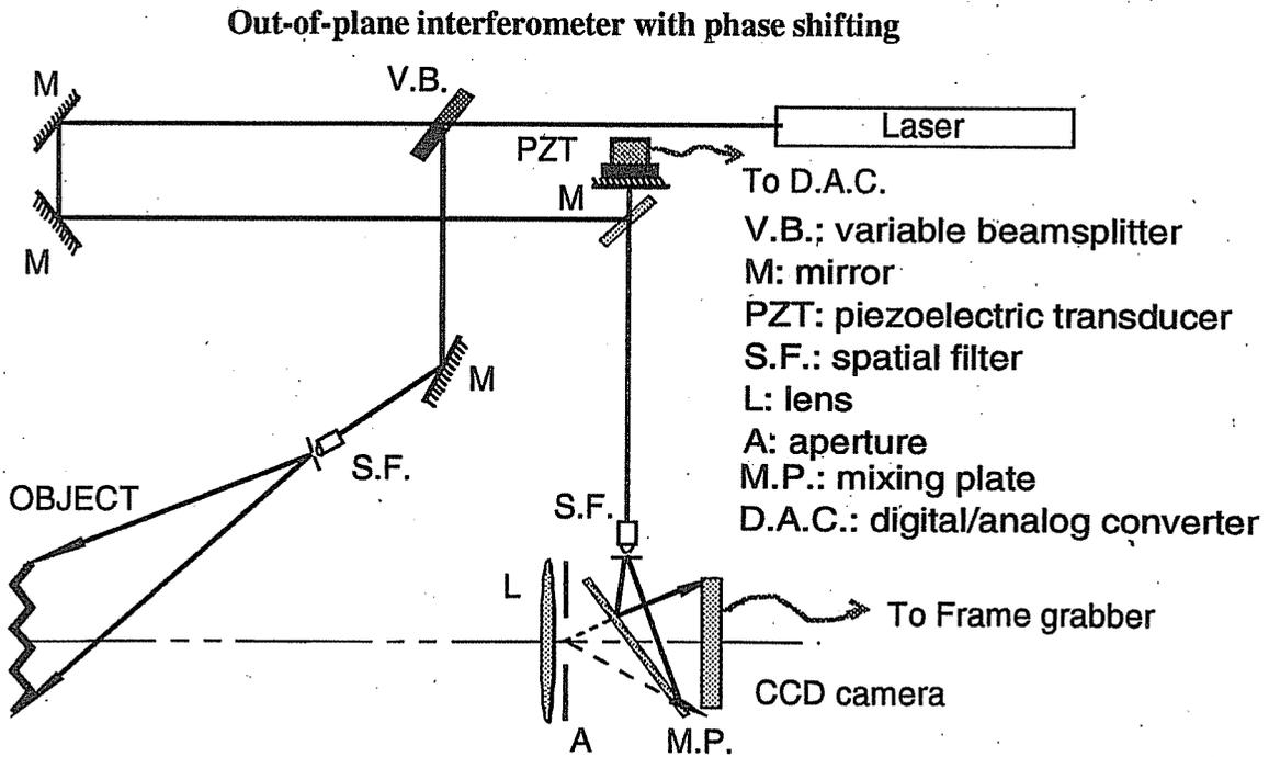
Fig. 4: DSPI measurement set-up
