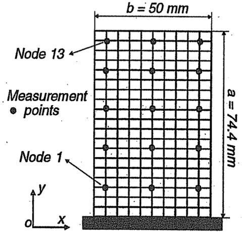
Fig. 3: FE model of the plate
