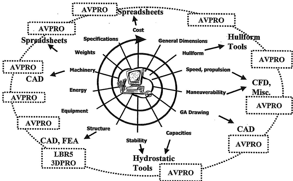
Figure 2-2 Software used in the design loop
