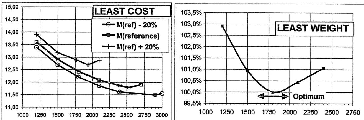
Figure 4-2: Sensitivity analysis: Cost and weight as a function of the web-frame spacing.
