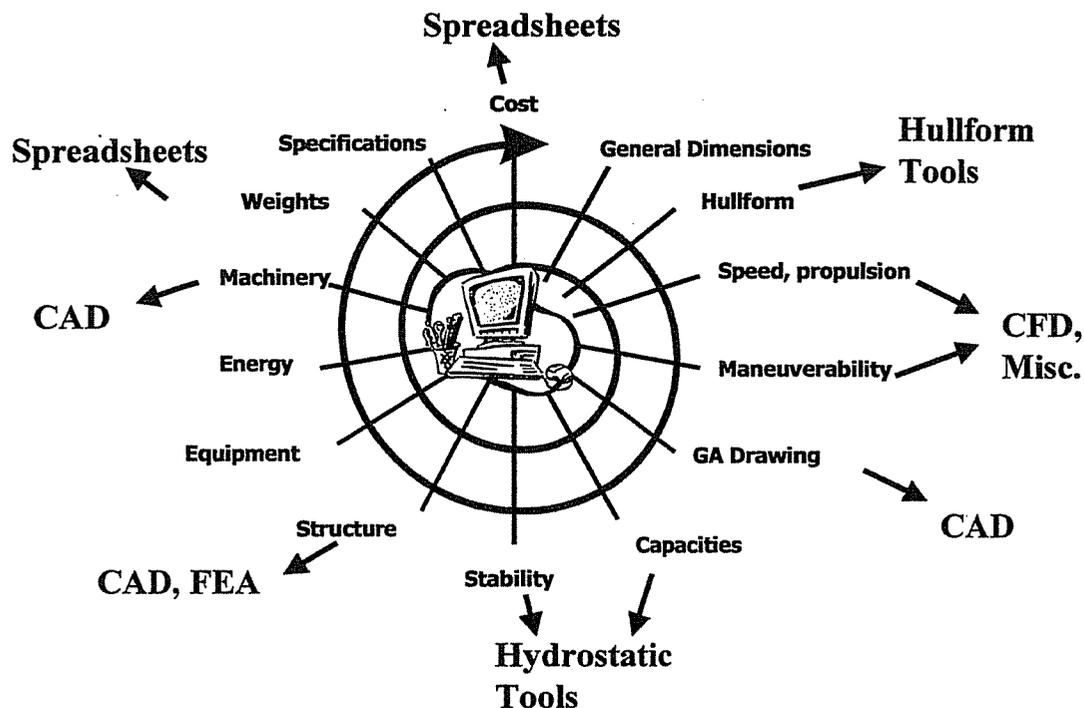
Figure 1-1 Software used in the design loop
