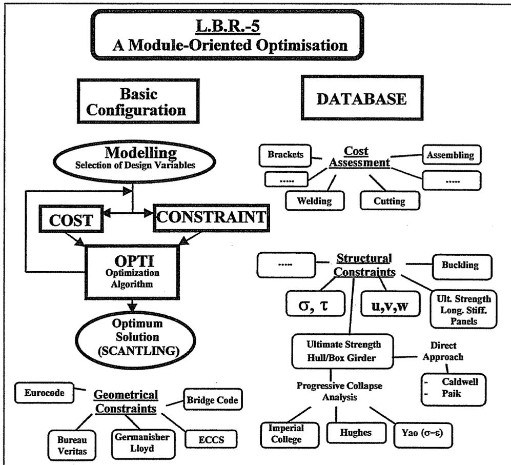
Figure 4-1 Basic configuration of the LBR-5 model and basic modules
