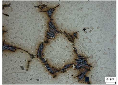
Figure 4c – M 2 C (Dark to blue) carbides at grain boundaries (Groesbeck etching, Aurora grade)
