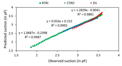
**Figure A1.** Correlation coefficient and RMSE between observed and fitted water suction from SWRC. Graph shows the linear correlation between predicted (from SWRC) and observed data. Slope = 1: perfect estimation, Slope > or < 1: over and underestimation.
