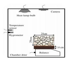
(a) Design of the drying chamber composed of the soil sample, camera, balance, heating bulb and sensors
