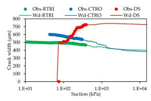
(**b**) Crack width as a function of suction. The big dots (Obs-) and line represent the observed and extrapolated data, respectively.
