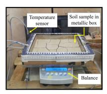
(**b**) Real photograph of the inside chamber showing the cracked sample in metallic box
