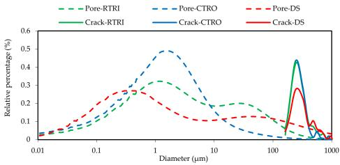
(a) Pore size distribution obtained from monomodal and bimodal fitting curves and the relative frequency of the crack width distribution for the undisturbed (NDS) and disturbed (DS) samples. The x-axis is set in logarithmic scale. Crack-RTRI/CTRO/DS: distribution of crack width in RTRI/CTRO/DS; Pore-RTRI/CTRO/DS: distribution of pores from SWRC in RTRI/CTRO/DS; RTRI: reduced-tillage-residue-in; CTRO: conventional-tillage-residue-out; DS: disturbed sample.
