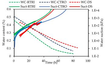
(c) Water content and extrapolated (line)/observed (dots) water suction change with time between RTRI, CTRO and DS
