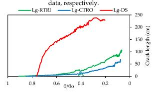
(c) Crack length progression with normalised water content ( $\theta/\theta o$ ) for DS and NDS, where  $\theta$  is the volumetric water content at time (t) and  $\theta o$  is the initial water content. The arrow points the critical water content for NDS.
