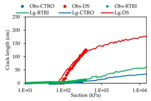
(a) Crack length as a function of the suction. The big dots and lines represent the observed and extrapolated
