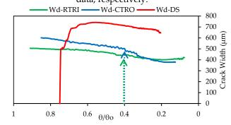
(d) Crack width progression with normalised water content ( $\theta/\theta$ o) for DS and NDS, where  $\theta$  is the volumetric water content at time (t) and  $\theta$ o is the initial water content. The arrow points the critical water content for NDS.
