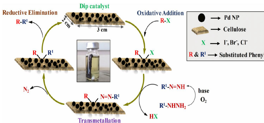
Figure 12. Mechanism proposed by Kempasiddaiah et al. for denitrogenative cross-coupling reactions [89].
