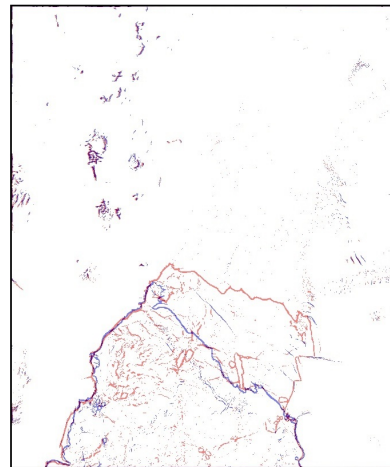
Fig. 5. Comparison between June 2017 (blue) and June 2020 (red). We observe that the calving front retreated by overall 20 kilometers, i.e. 20 meters per day on average (the retreat is far from continuous but rather results from sudden large calving events).
