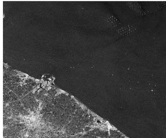
Figure 1. Double bounce effect, revealing anthropogenic structures: buildings, offshore wind turbines and boats (illustration from Sentinel-1 over the Belgian coast)
